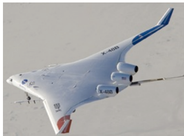
Figure 1. The Boeing X-48B Blended Wing Body, shown in flight near the NASA Dryden Flight Research Center.
