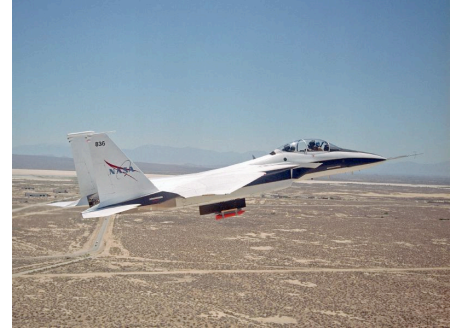
Figure 1. One of the NASA Dryden Flight Research Center F-15B aircraft, tail number 836, shown in flight with the Propulsion Flight Test Fixture pylon.
